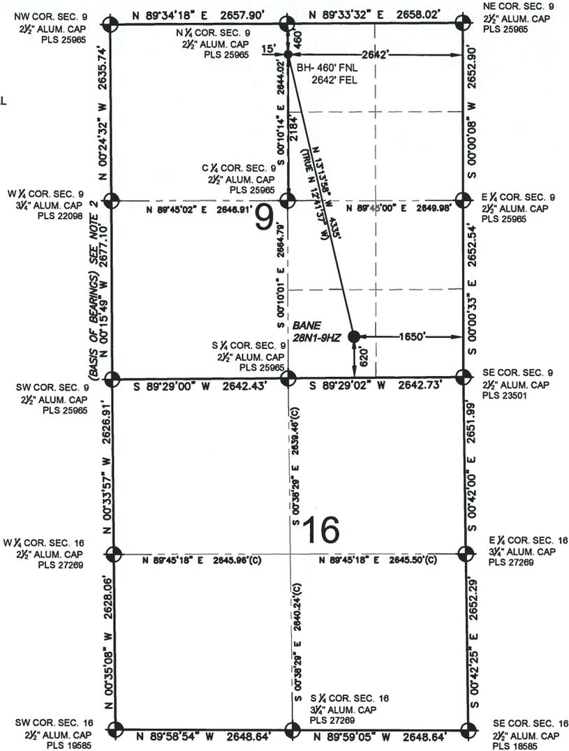
**WELL BANE 28N1-9HZ TO BE LOCATED 620' FSL AND 1650' FEL**
