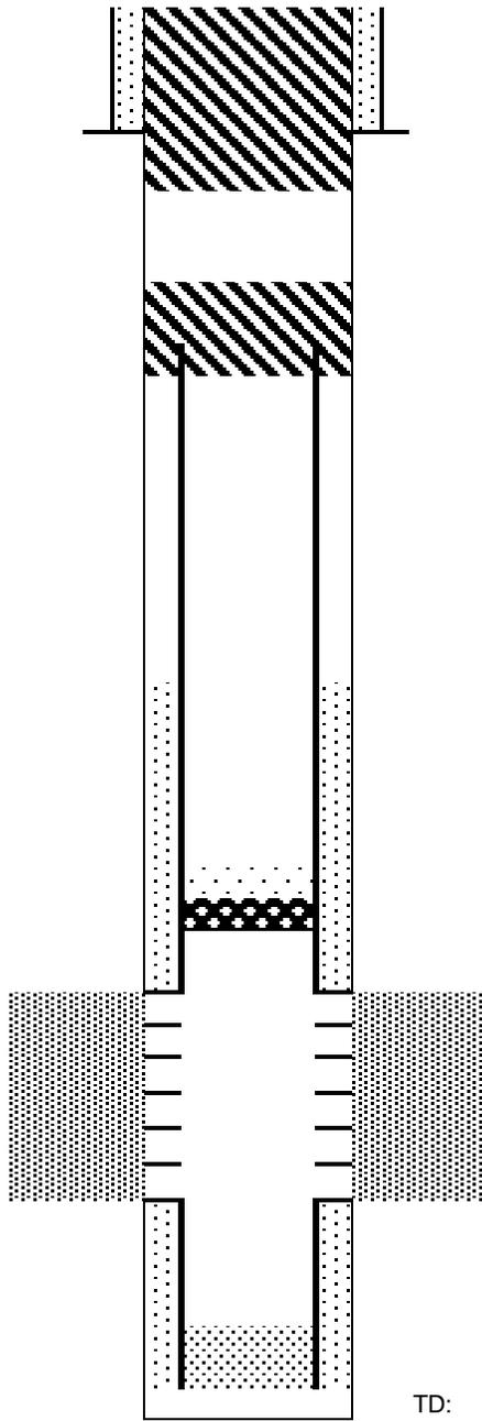
Cut surface casing off 6'-8' below surface.
