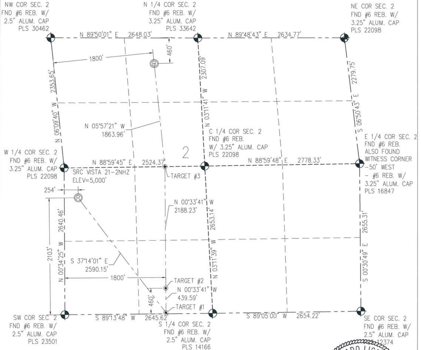
IN ACCORDANCE WITH A REQUEST FROM CRAIG RASMUSON - SYNERGY RESOURCES, BASELINE ENGINEERING CORP. HAS DETERMINED THE LOCATION OF THE SRC VISTA 21-2NHZ TO BE 2103' FSL AND 254' FWL, AS MEASURED AT NINETY (90) DEGREES FROM THE SECTION LINE OF SECTION 2, TOWNSHIP 4 NORTH, RANGE 68 WEST AND THE BOTTOM HOLE LOCATION TO BE 460' FNL AND 1800' FWL OF SECTION 2, TOWNSHIP 4 NORTH, RANGE 68 WEST, 6TH PRINCIPAL MERIDIAN, WELD COUNTY, COLORADO.
