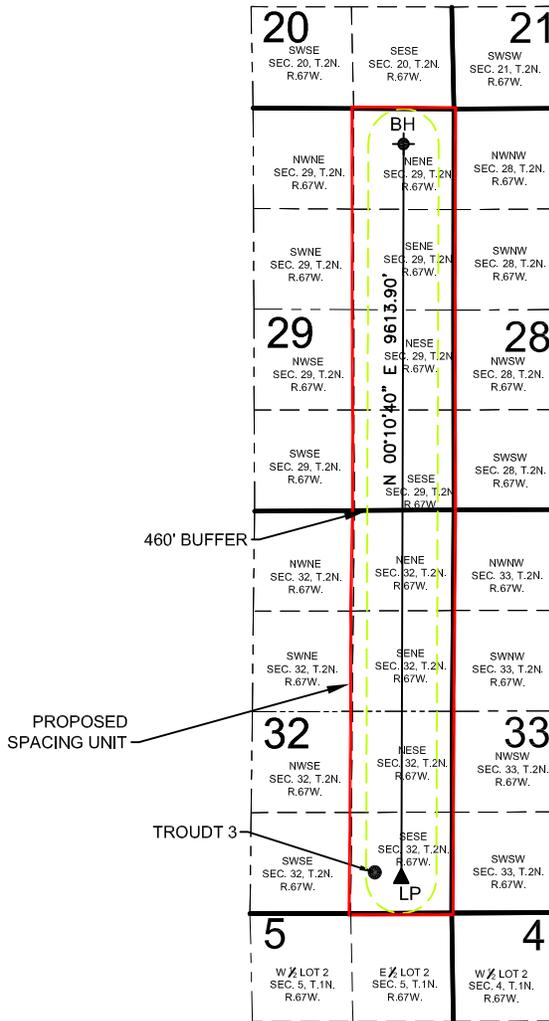
WELL TROUDT 3 TO BE LOCATED 537' FSL AND 1007' FEL, SEC. 32, T2N, R67W
