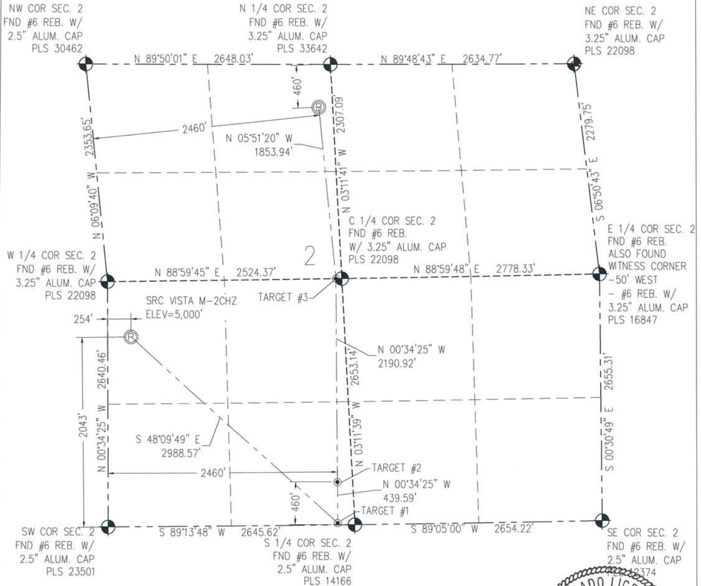
IN ACCORDANCE WITH A REQUEST FROM CRAIG RASMUSON - SYNERGY RESOURCES, BASELINE ENGINEERING CORP. HAS DETERMINED THE LOCATION OF THE SRC VISTA M-2CHZ TO BE 2043' FSL AND 254' FWL, AS MEASURED AT NINETY (90) DEGREES FROM THE SECTION LINE OF SECTION 2, TOWNSHIP 4 NORTH, RANGE 68 WEST AND THE BOTTOM HOLE LOCATION TO BE 460' FNL AND 2460' FWL OF SECTION 2, TOWNSHIP 4 NORTH, RANGE 68 WEST, 6TH PRINCIPAL MERIDIAN, WELD COUNTY, COLORADO.
