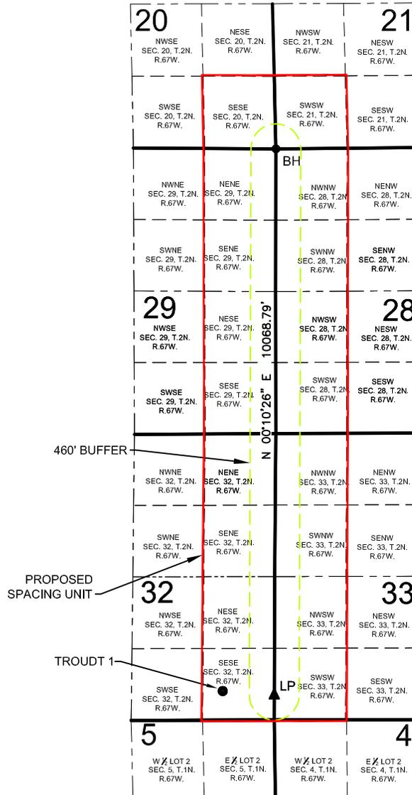
WELL TROUDT 1 TO BE LOCATED 537' FSL AND 951' FEL, SEC. 32, T2N, R67W
