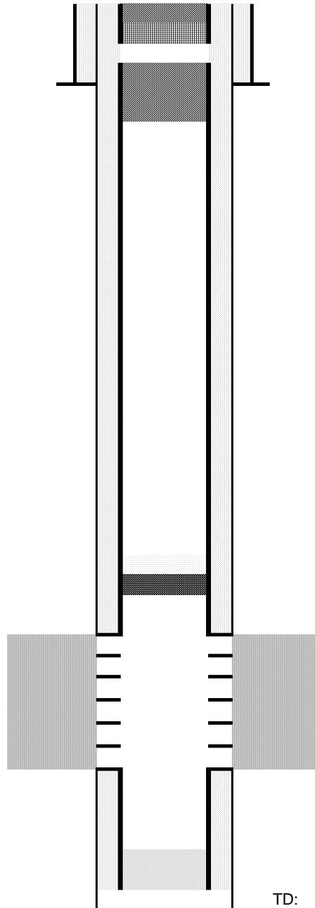
**Cut surface casing off 6'-8' below surface.**
