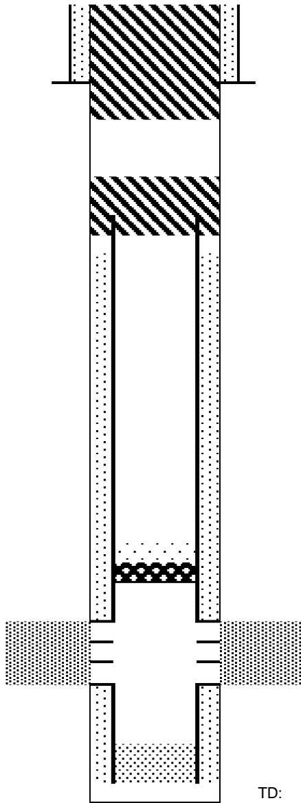
Cut surface casing off 6'-8' below surface.
