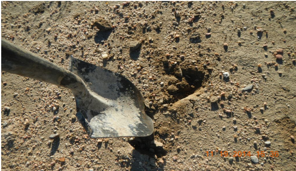
photo 9: Shovel could not break through soil surface indicating soil compaction.
