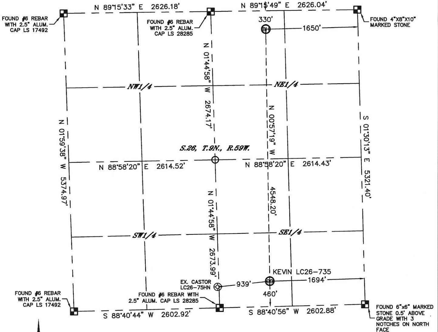
In accordance with a request from Cody Ball with Noble Energy Inc. Lat40°, Inc. has determined the surface location of the KEVIN LC26-735 to be 460' from the SOUTH line and 1694' from the EAST line and the bottom hole to be 330' from the NORTH line and 1650' from the EAST line as measured at right angles from the section lines of Section 26, Township 9 North, Range 59 West of the Sixth Principal Meridian, County of Weld, State of Colorado.
