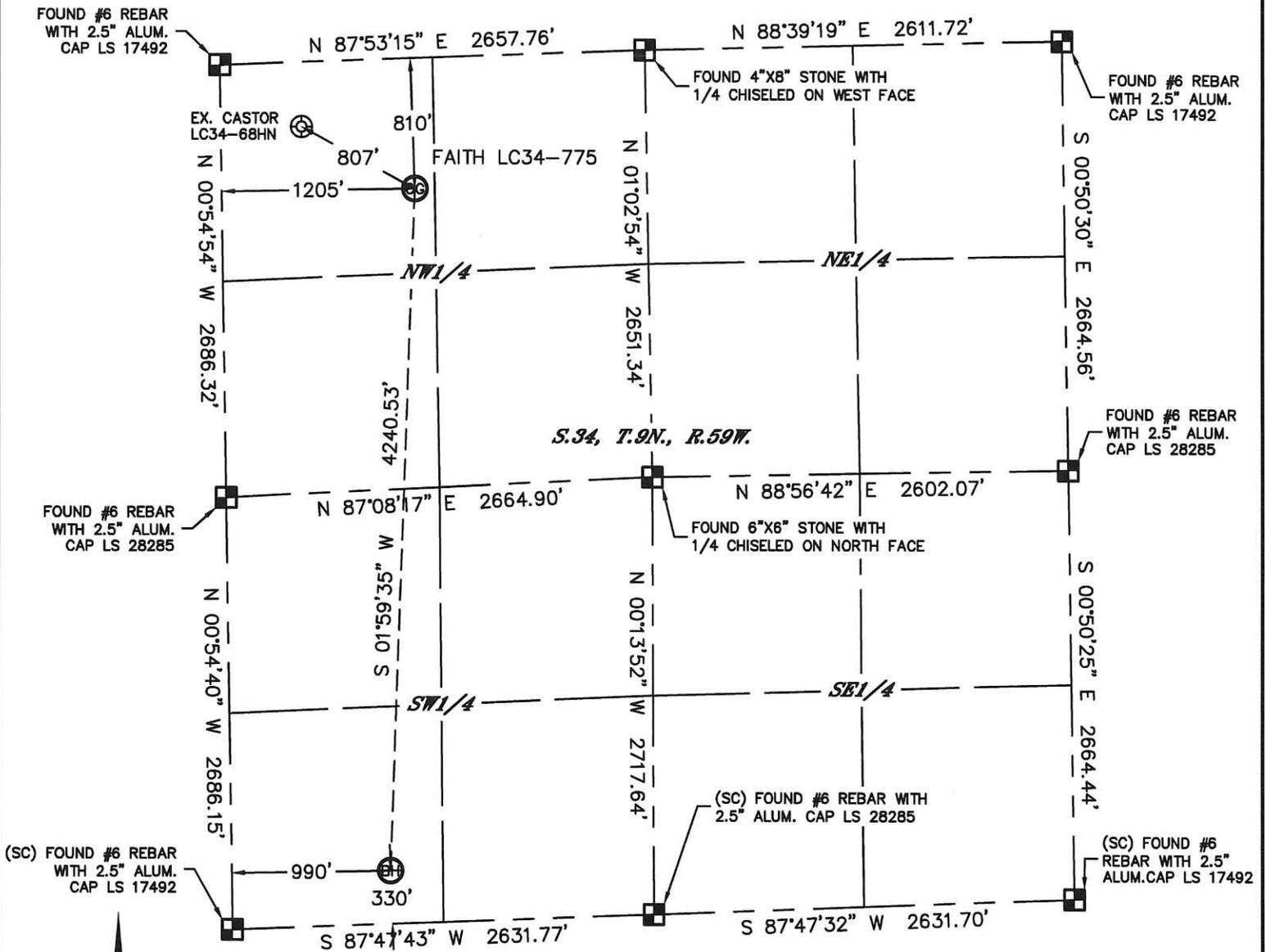
In accordance with a request from Brian James with Noble Energy Inc. Lat40°, Inc. has determined the surface location of the FAITH LC34-775 to be 810' from the NORTH line and 1205' from the WEST line and the bottom hole to be 330' from the SOUTH line and 990' from the WEST line as measured at right angles from the section lines of Section 34, Township 9 North, Range 59 West of the Sixth Principal Meridian, County of Weld, State of Colorado.
