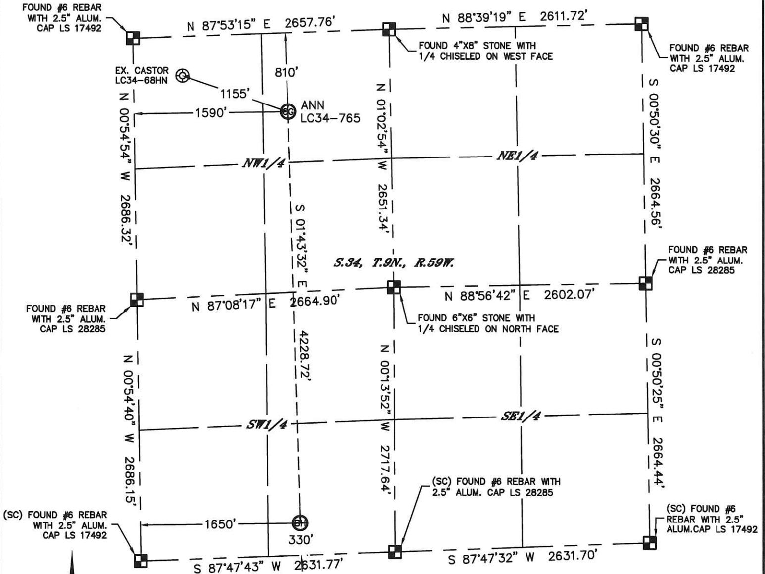
In accordance with a request from Brian James with Noble Energy Inc. Lat40°, Inc. has determined the surface location of the ANN LC34-765 to be 810' from the NORTH line and 1590' from the WEST line and the bottom hole to be 330' from the SOUTH line and 1650' from the WEST line as measured at right angles from the section lines of Section 34, Township 9 North, Range 59 West of the Sixth Principal Meridian, County of Weld, State of Colorado.
