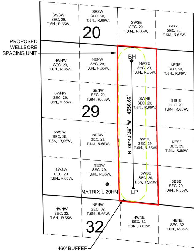
**WELL MATRIX L-29HN TO BE LOCATED 520' FSL AND 2212' FWL, SEC. 29, T6N, R65W**
