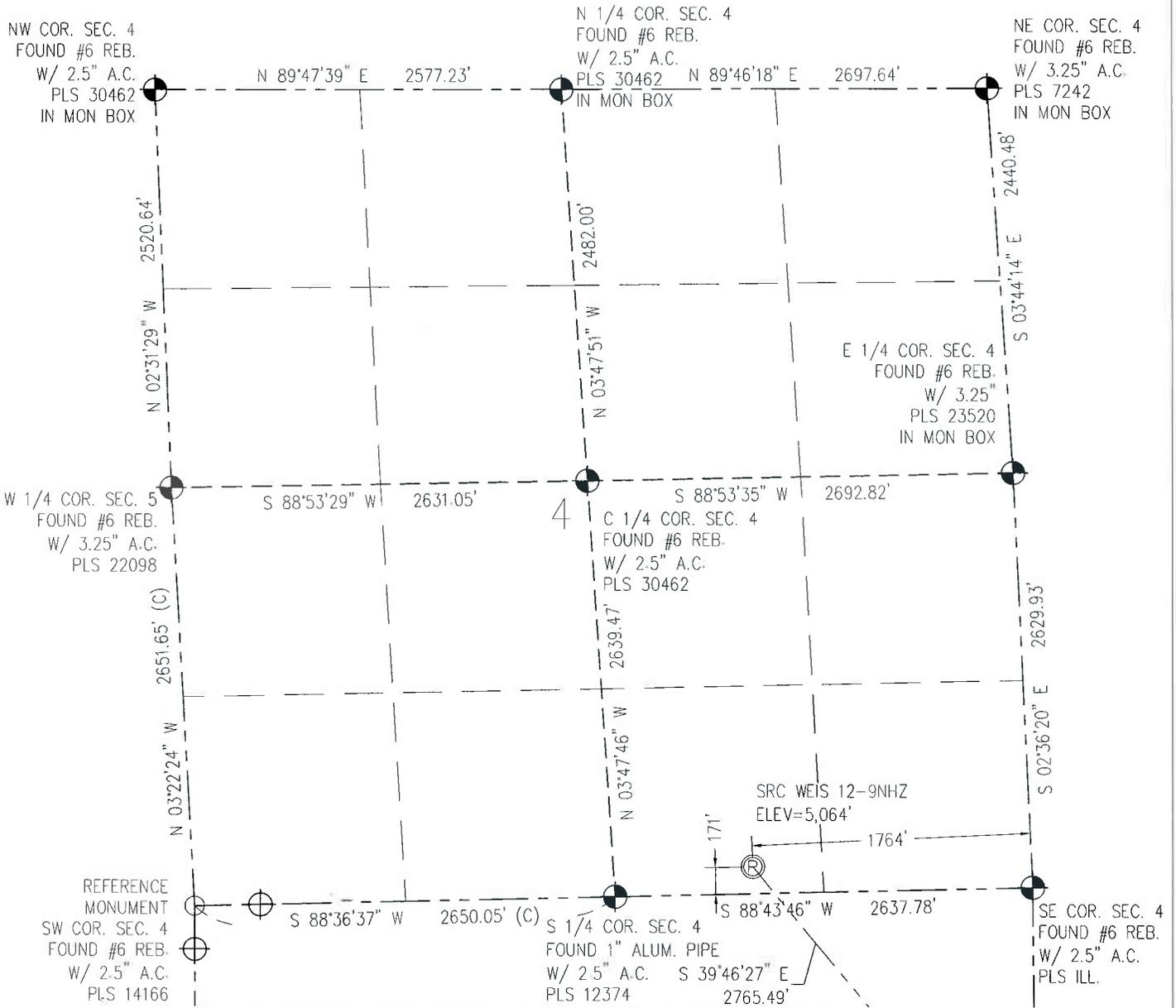
IN ACCORDANCE WITH A REQUEST FROM CRAIG RASMUSON - SYNERGY RESOURCES, BASELINE ENGINEERING CORP HAS DETERMINED THE LOCATION OF THE SRC WEIS 12-9NHZ TO BE 171' FSL AND 1764' FEL, AS MEASURED AT NINETY (90) DEGREES FROM THE SECTION LINE OF SECTION 4, TOWNSHIP 4 NORTH, RANGE 68 WEST AND THE BOTTOM HOLE LOCATION TO BE 460' FWL AND 1970' FNL OF SECTION 9, TOWNSHIP 4 NORTH, RANGE 68 WEST, 6TH PRINCIPAL MERIDIAN, WELD COUNTY, COLORADO.
