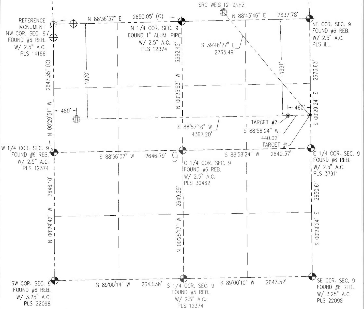
**N** IN ACCORDANCE WITH A REQUEST FROM CRAIG RASMUSON - SYNERGY RESOURCES, BASELINE ENGINEERING CORP. HAS DETERMINED THE LOCATION OF THE SRC WEIS 12-9NHZ TO BE 171' FSL AND 1764' FEL, AS MEASURED AT NINETY (90) DEGREES FROM THE SECTION LINE OF SECTION 4, TOWNSHIP 4 NORTH, RANGE 68 WEST AND THE BOTTOM HOLE LOCATION TO BE 460' FWL AND 1970' FNL OF SECTION 9, TOWNSHIP 4 NORTH, RANGE 68 WEST, 6TH PRINCIPAL MERIDIAN, WELD COUNTY, COLORADO.
