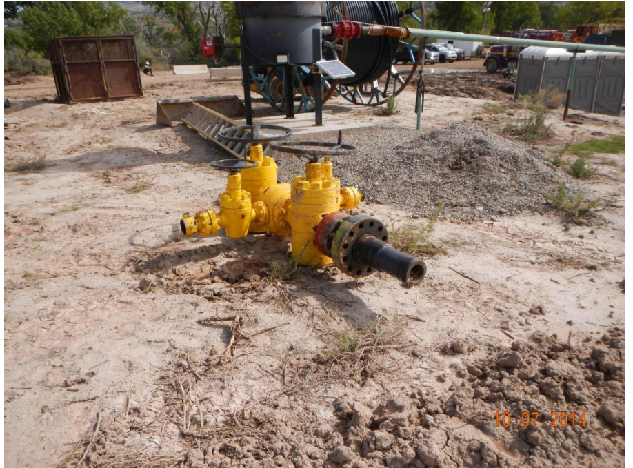
Frac tree with mandrel stored off location.
