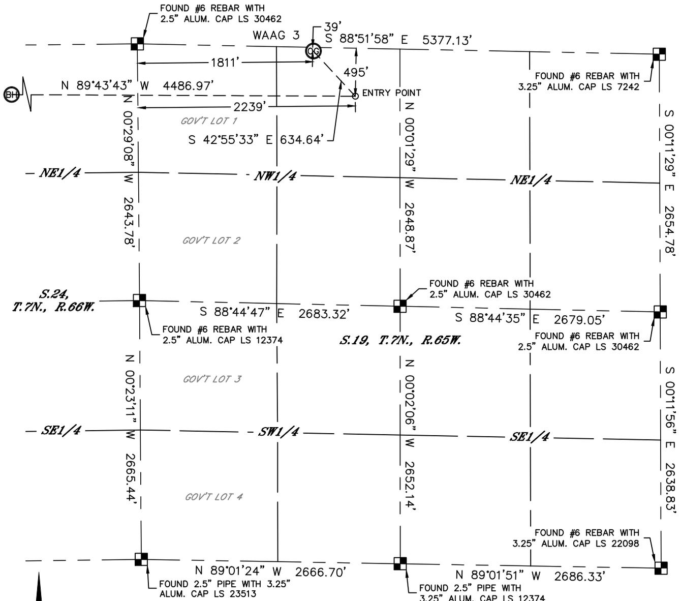
In accordance with a request from Derek Petrie with EXTRACTION OIL & GAS Lat40°, Inc. has determined the surface location of the WAAG 3 to be 39' from the NORTH line and 11811' from the WEST line of Section 19, Township 7 North, Range 65 West and the bottom hole to be 495' from the NORTH line and 2247' from the EAST line as measured at right angles from the section lines of Section 24, Township 7 North, Range 66 West of the Sixth Principal Meridian, County of Weld, State of Colorado.
