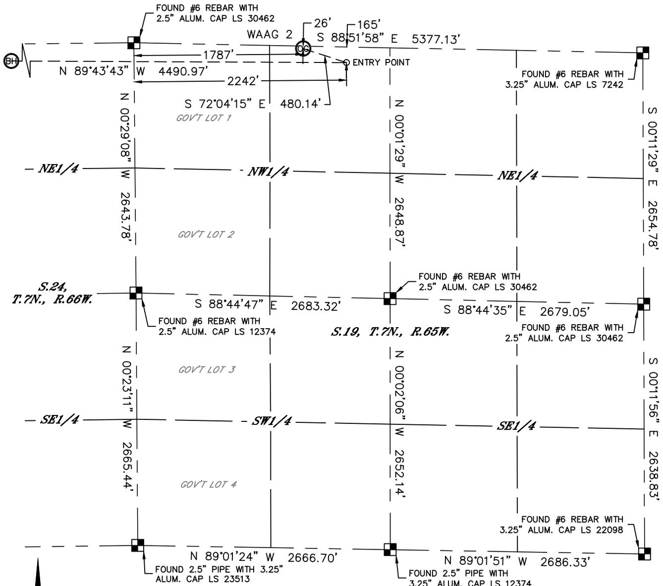
In accordance with a request from Derek Petrie with EXTRACTION OIL & GAS Lat40°, Inc. has determined the surface location of the WAAG 2 to be 26' from the NORTH line and 1787' from the WEST line of Section 19, Township 7 North, Range 65 West and the bottom hole to be 165' from the NORTH line and 2248' from the EAST line as measured at right angles from the section lines of Section 24, Township 7 North, Range 66 West of the Sixth Principal Meridian, County of Weld, State of Colorado.
