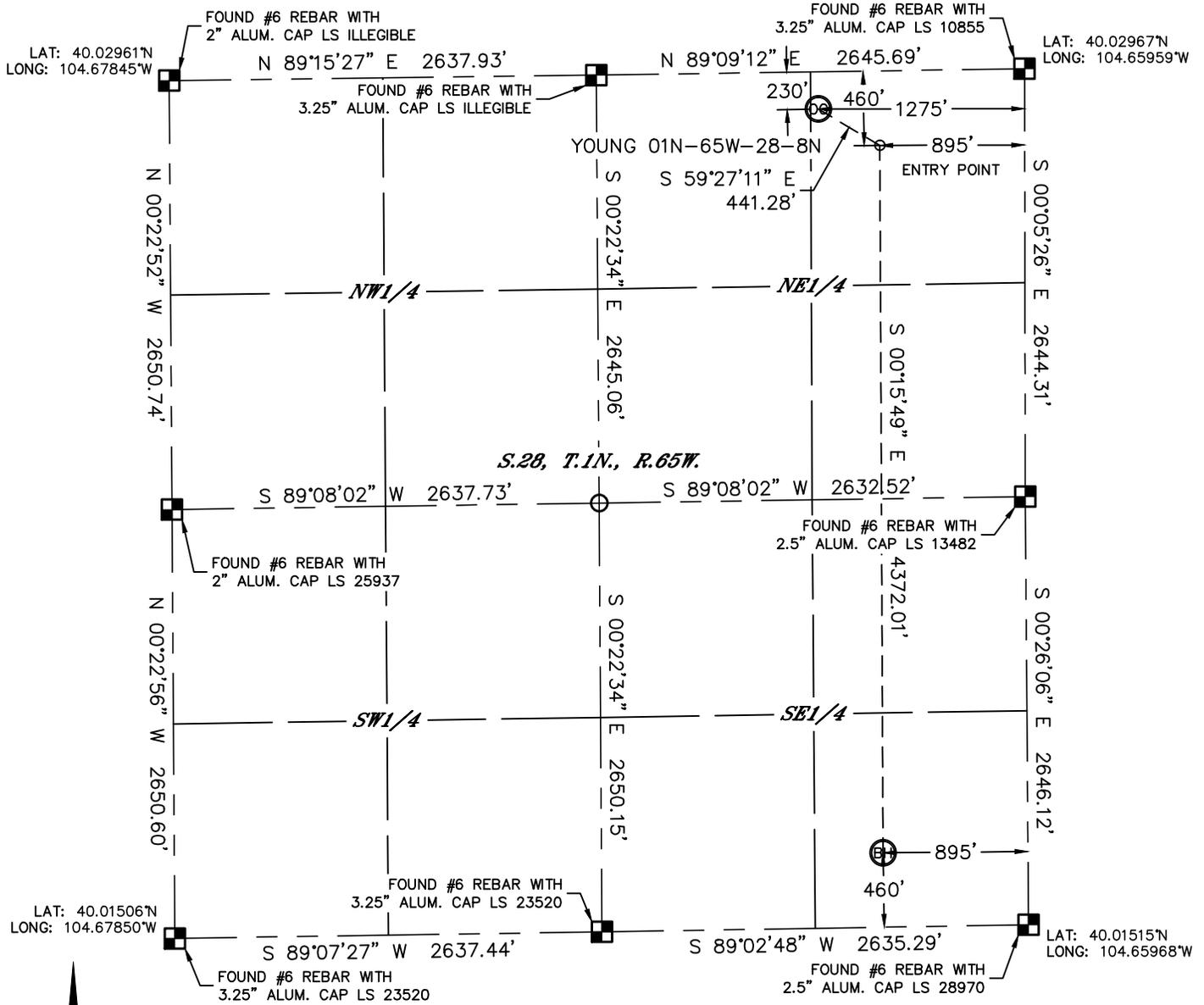
In accordance with a request from Arthur Beecher with VERDAD OIL & GAS CORPORATION Lat40°, Inc. has determined the surface location of the YOUNG 01N-65W-28-8N to be 230' from the NORTH line and 1275' from the EAST line and the bottom hole to be 460' from the SOUTH line and 895' from the EAST line as measured at right angles from the section lines of Section 28, Township 1 North, Range 65 West of the Sixth Principal Meridian, County of Weld, State of Colorado.
