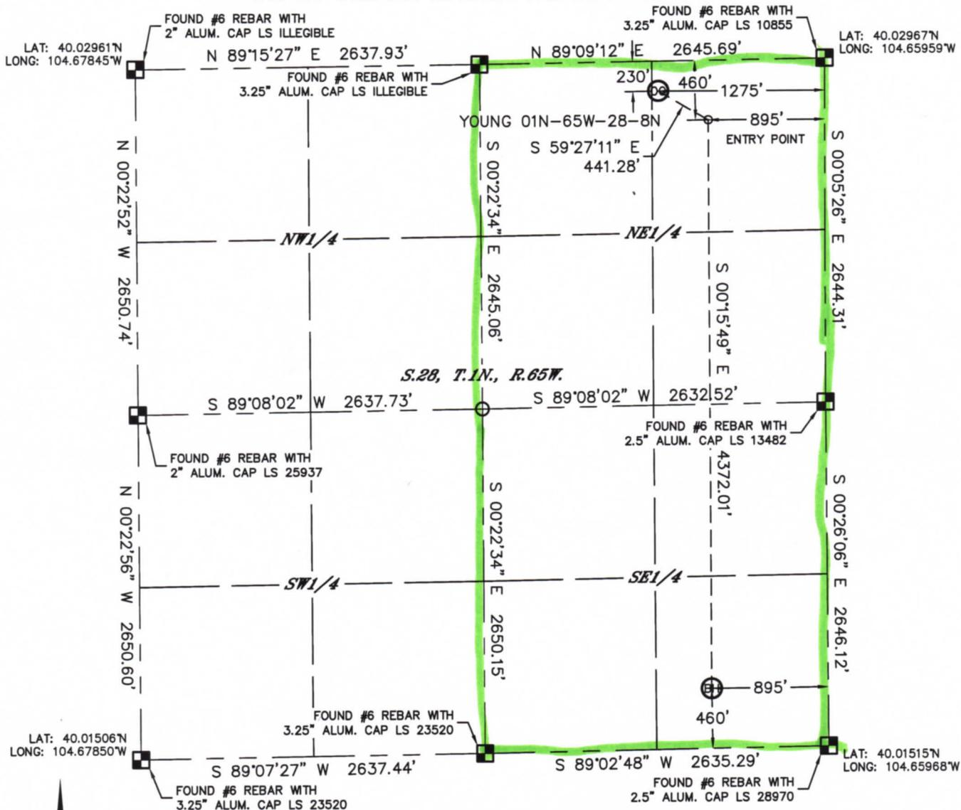
In accordance with a request from Arthur Beecher with VERDAD OIL & GAS CORPORATION Lat40°, Inc. has determined the surface location of the YOUNG 01N-65W-28-8N to be 230' from the NORTH line and 1275' from the EAST line and the bottom hole to be 460' from the SOUTH line and 895' from the EAST line as measured at right angles from the section lines of Section 28, Township 1 North, Range 65 West of the Sixth Principal Meridian, County of Weld, State of Colorado.
