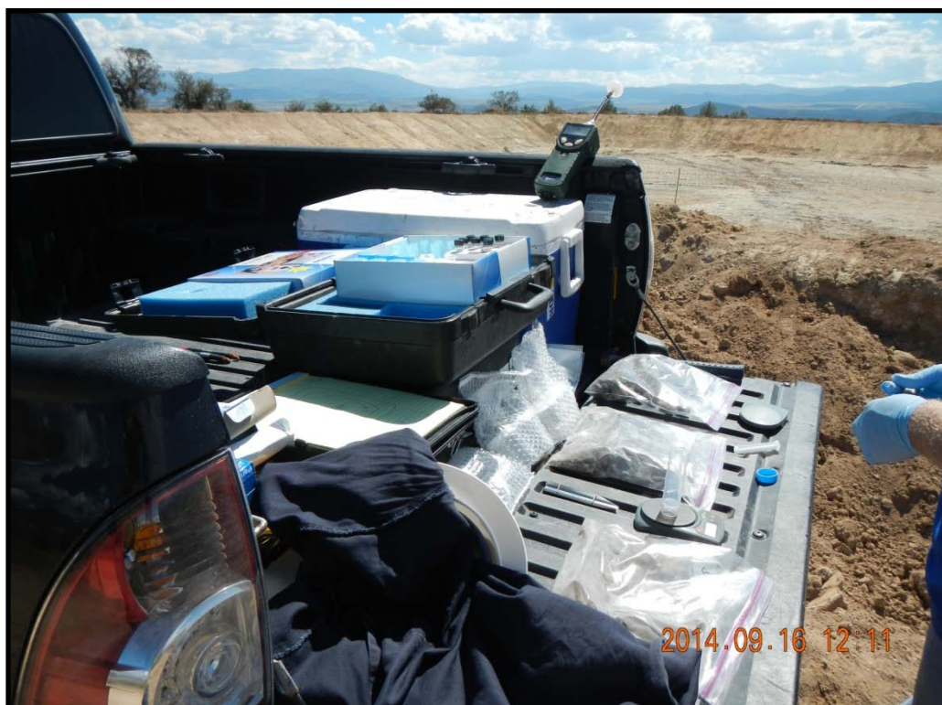
Using PID and Petroflag to screen soil samples for volatile hydrocarbons.
