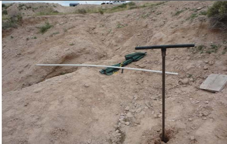
**Subject:** Photograph shows the location of the hand auger hole and 1" diameter by ten feet PVC casing for piezometer, PZ-1.
