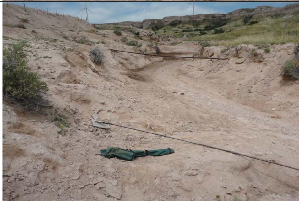
**Subject:** Photograph shows the piezometer, PZ-1, and hand auger after being set and the elevation above the base of the drainage. The piezometer remained dry during the site visit.
