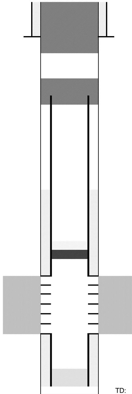
Cut surface casing off 6'-8' below surface.
