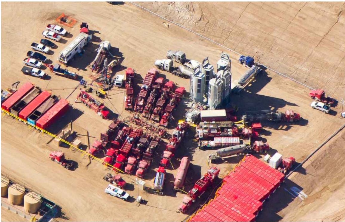
TEMPORARY COMPLETION EQUIPMENT EXAMPLE CONFIGURATION ESTIMATED DURATION ON-SITE: 2 DAYS PER WELL
