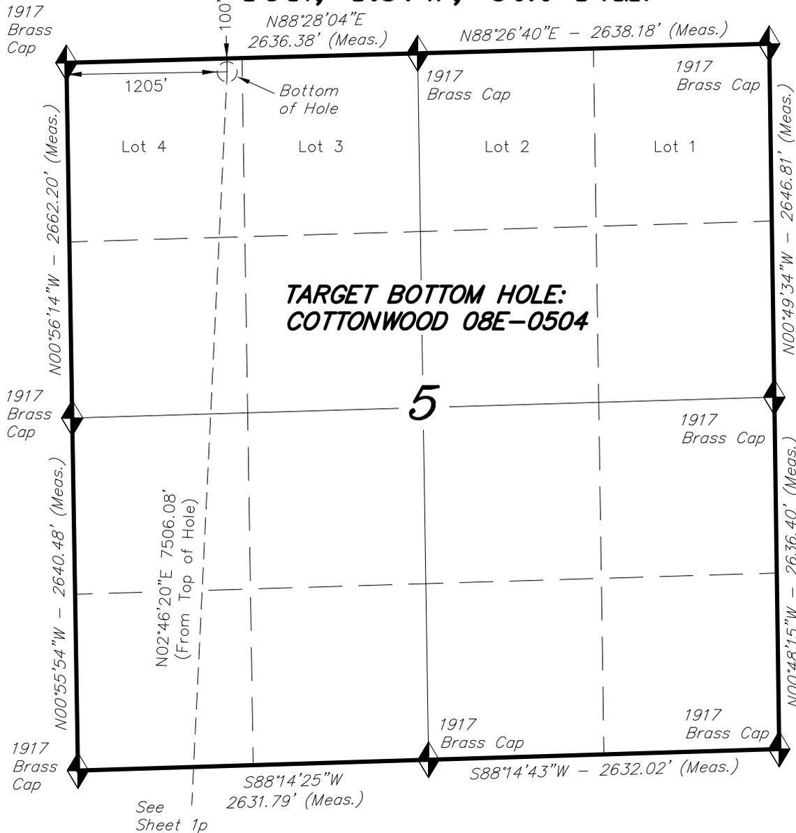
TARGET BOTTOM HOLE, COTTONWOOD 08E-0504, LOCATED AS SHOWN IN THE NW 1/4 NW 1/4 (LOT 4) OF SECTION 5, T9N, R57W, 6th P.M. WELD COUNTY, COLORADO.
