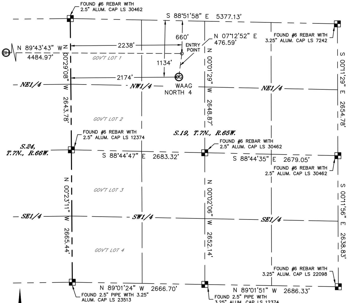
In accordance with a request from Derek Petrie with EXTRACTION OIL & GAS Lat40°, Inc. has determined the surface location of the WAAG NORTH 4 to be 1134' from the NORTH line and 2174' from the WEST line of Section 19, Township 7 North, Range 65 West and the bottom hole to be 660' from the NORTH line and 2246' from the EAST line as measured at right angles from the section lines of Section 24, Township 7 North, Range 66 West of the Sixth Principal Meridian, County of Weld, State of Colorado.
