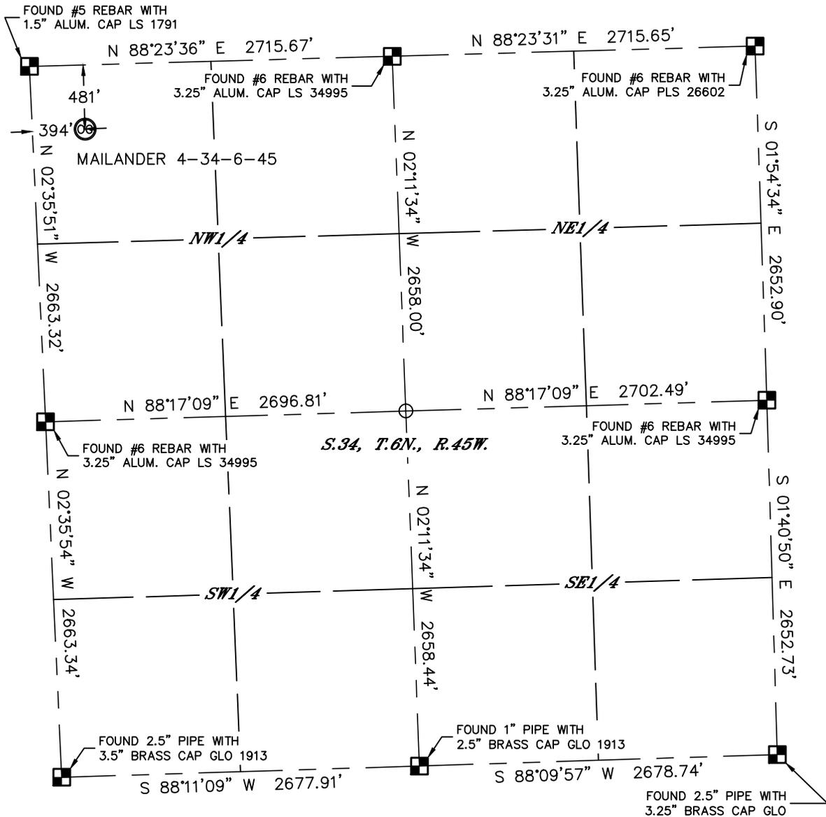
In accordance with a request from Michelle Lewis with OMIMEX PETROLEUM, INC. Lat40°, Inc. has determined the surface location of the MAILANDER 4-34-6-45 to be 481' from the NORTH line and 394' from the WEST line as measured at right angles from the section lines of Section 34, Township 6 North, Range 45 West of the Sixth Principal Meridian, County of Phillips, State of Colorado.
