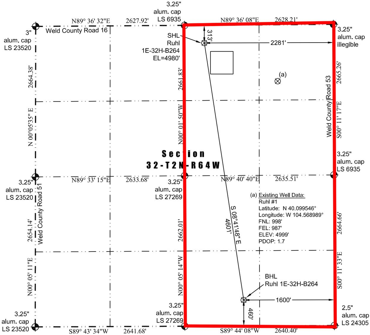
In accordance with a request from Jay Knutson of EnCana Oil & Gas (USA) Inc., Washburn Land Surveying, LLC has determined the location of the **Ruhl 1E-32H-B264** well site to be SHL: 313' FNL and 2281' FEL, (BHL: 460' FSL and 1600' FEL), as measured at ninety (90) degrees from the section lines of Section 32, Township 2 North, Range 64 West of the 6th Principal Meridian, Weld County Colorado.
