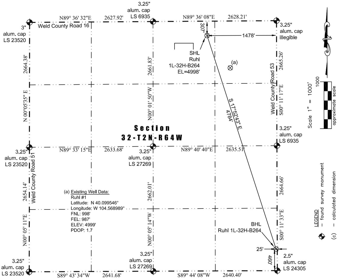
In accordance with a request from Jay Knutson of EnCana Oil & Gas (USA) Inc., Washburn Land Surveying, LLC has determined the location of the **Ruhl 1L-32H-B264** well site to be SHL: 307' FNL and 1478' FEL, (BHL: 460' FSL and 25' FEL), as measured at ninety (90) degrees from the section lines of Section 32, Township 2 North, Range 64 West of the 6th Principal Meridian, Weld County Colorado.
