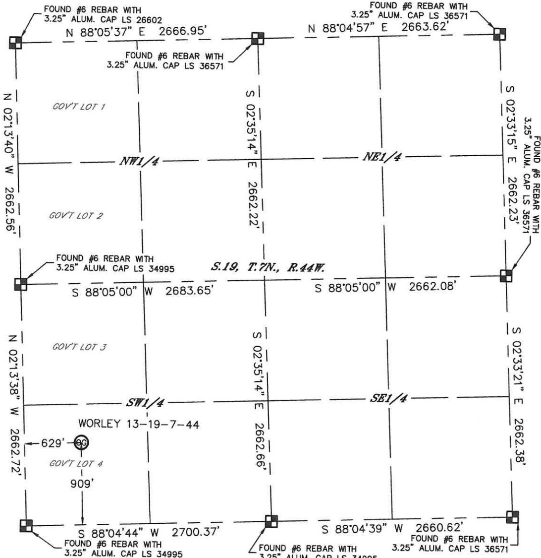
In accordance with a request from Michelle Lewis with Omimex Petroleum, Inc. Lat40°, Inc. has determined the surface location of the WORLEY 13-19-7-44 to be 909' from the SOUTH line and 629' from the WEST line as measured at right angles from the section lines of Section 19, Township 7 North, Range 44 West of the Sixth Principal Meridian, County of Phillips, State of Colorado.
