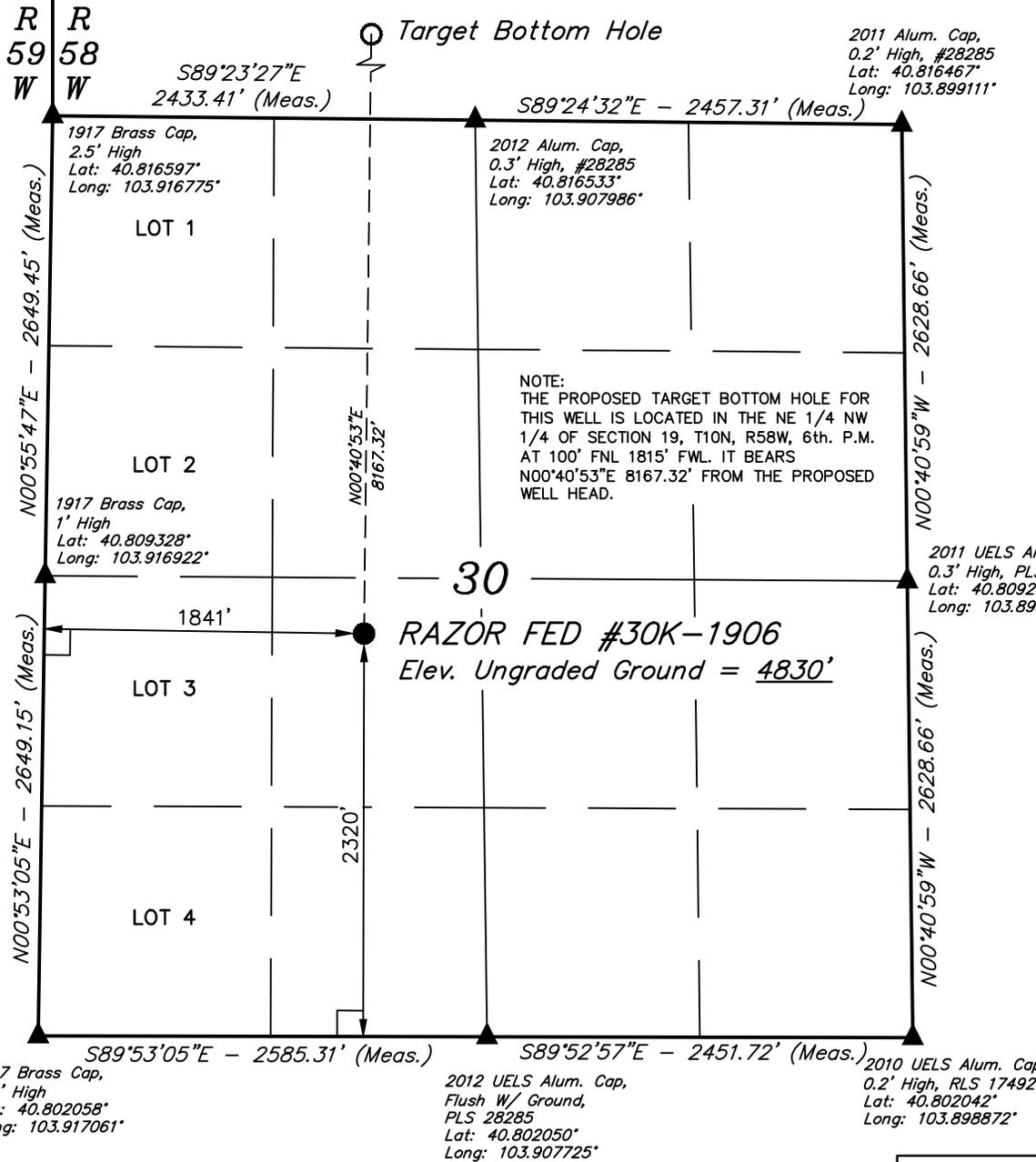
Well location, RAZOR FED #30K-1906, (SURFACE LOCATION), located as shown in the NE 1/4 SW 1/4 of Section 30, T10N, R58W, 6th. P.M., Weld County, Colorado.
