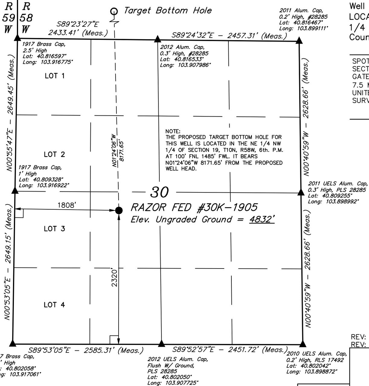
Well location, RAZOR FED #30K-1905, (SURFACE LOCATION), located as shown in the NE 1/4 SW 1/4 of Section 30, T10N, R58W, 6th. P.M., Weld County, Colorado.
