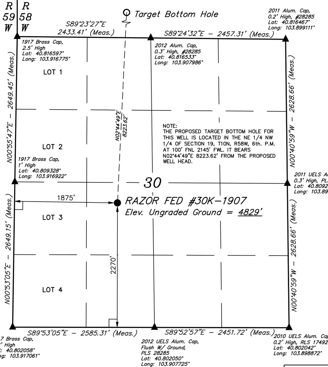
Well location, RAZOR FED #30K-1907, (SURFACE LOCATION), located as shown in the NE 1/4 SW 1/4 of Section 30, T10N, R58W, 6th. P.M., Weld County, Colorado.
