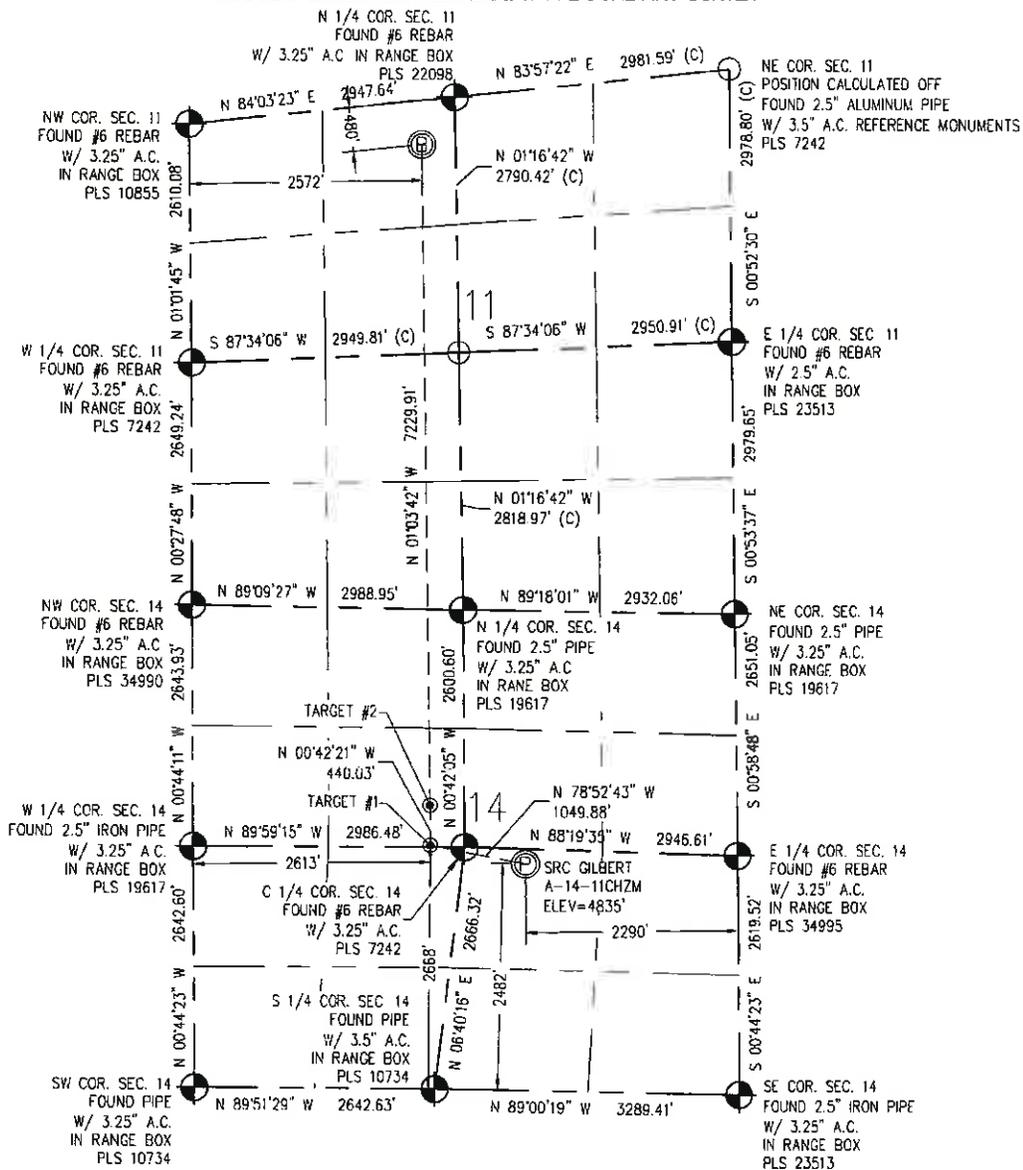
IN ACCORDANCE WITH A REQUEST FROM CRAIG RASMUSON - SYNERGY RESOURCES, BASELINE ENGINEERING CORP HAS DETERMINED THE LOCATION OF THE SRC GILBERT A-14-11CHZM TO BE 2,482' FSL AND 2,290' FEL, AS MEASURED AT NINETY (90) DEGREES FROM THE SECTION LINE OF SECTION 14, TOWNSHIP 5 NORTH, RANGE 66 WEST AND THE BOTTOM HOLE LOCATION TO BE 480' FNL AND 2,572' FWL OF SECTION 11, TOWNSHIP 5 NORTH, RANGE 66 WEST, 6TH PRINCIPAL MERIDIAN, WELD COUNTY, COLORADO.
