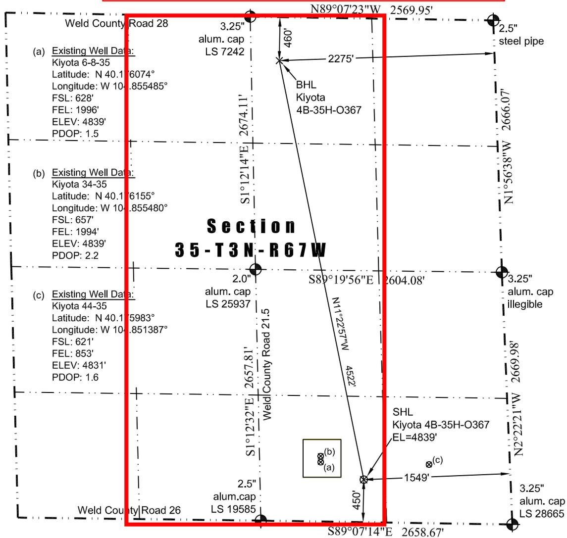
In accordance with a request from Jay Knutson of EnCana Oil & Gas (USA) Inc., Washburn Land Surveying, LLC has determined the location of the **Kiyota 4B-35H-O367** well site to be SHL: 450' FSL and 1549' FEL, (BHL: 460' FNL and 2275' FEL), as measured at ninety (90) degrees from the section lines of Section 35, Township 3 North, Range 67 West of the 6th Principal Meridian, Weld County Colorado.
