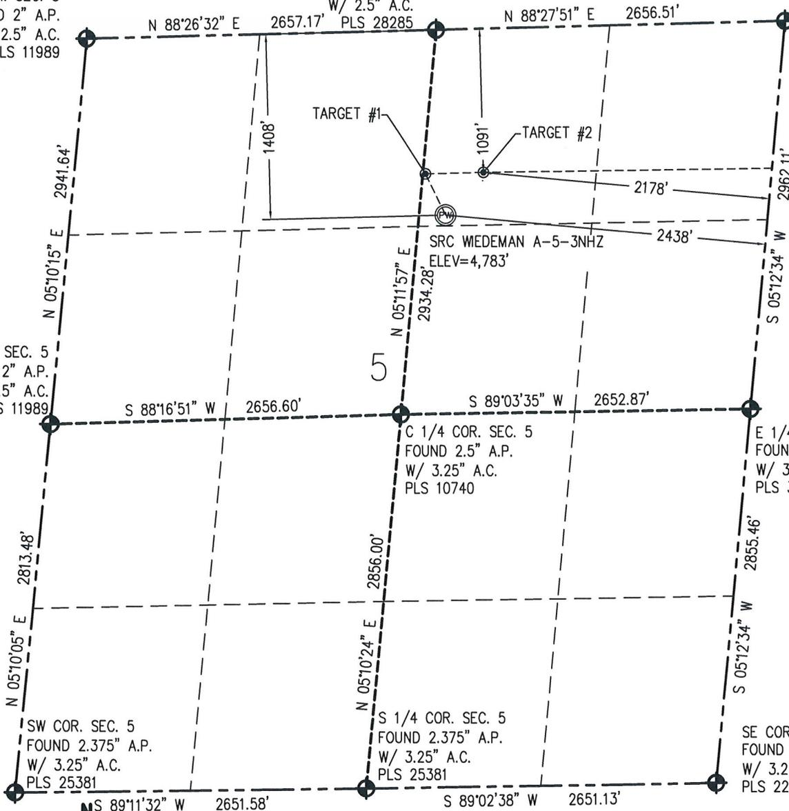
IN ACCORDANCE WITH A REQUEST FROM CRAIG RASMUSON - SYNERGY RESOURCES, BASELINE ENGINEERING CORP. HAS DETERMINED THE LOCATION OF THE SRC WIEDEMAN A-5-3NHZ TO BE 1408' FNL AND 2438' FEL, AS MEASURED AT NINETY (90) DEGREES FROM THE SECTION LINE OF SECTION 5, TOWNSHIP 5 NORTH, RANGE 66 WEST AND THE BOTTOM HOLE LOCATION TO BE 1091' FNL AND 2149' FWL OF SECTION 3, TOWNSHIP 5 NORTH, RANGE 66 WEST, 6TH PRINCIPAL MERIDIAN, WELD COUNTY, COLORADO.
