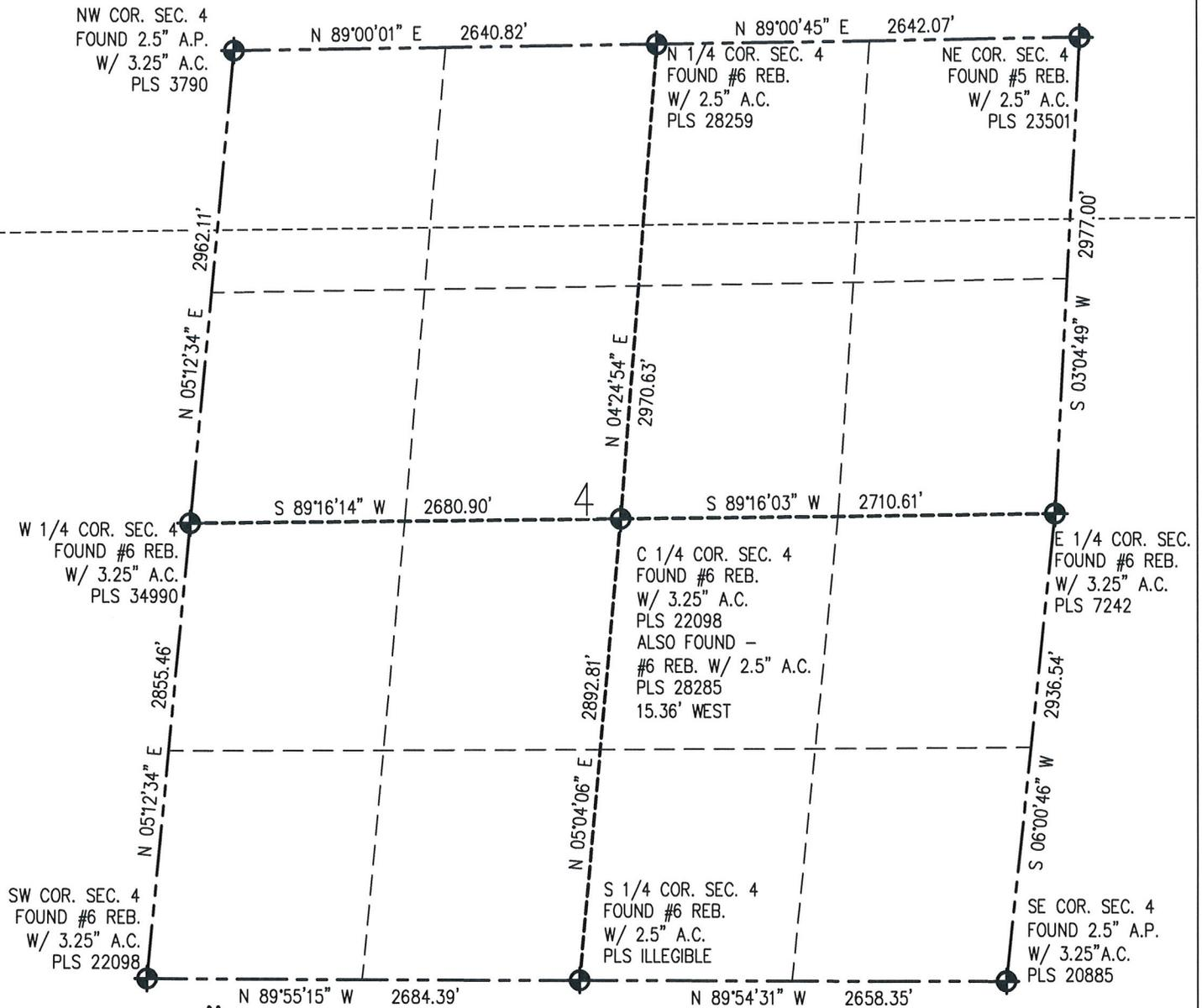
IN ACCORDANCE WITH A REQUEST FROM CRAIG RASMUSON - SYNERGY RESOURCES, BASELINE ENGINEERING CORP. HAS DETERMINED THE LOCATION OF THE SRC WEDEMAN A-5-3NHZ 1408' FNL AND 2438' FEL, AS MEASURED AT NINETY (90) DEGREES FROM THE SECTION LINE OF SECTION 5, TOWNSHIP 5 NORTH, RANGE 66 WEST AND THE BOTTOM HOLE LOCATION TO BE 1091' FNL AND 2149' FWL OF SECTION 3, TOWNSHIP 5 NORTH, RANGE 66 WEST, 6TH PRINCIPAL MERIDIAN, WELD COUNTY, COLORADO.
