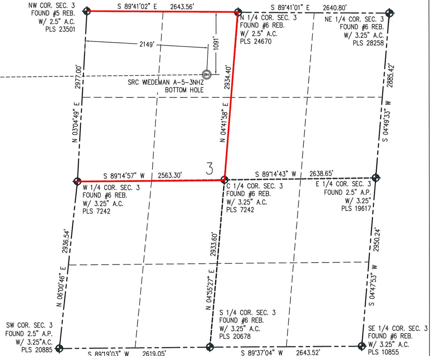
IN ACCORDANCE WITH A REQUEST FROM CRAIG RASMUSON - SYNERGY RESOURCES, BASELINE ENGINEERING CORP. HAS DETERMINED THE LOCATION OF THE SRC WEDEMAN A-5-3NHZ TO BE 1408' FNL AND 2438' FWL, AS MEASURED AT NINETY (90) DEGREES FROM THE SECTION LINE OF SECTION 5, TOWNSHIP 5 NORTH, RANGE 66 WEST AND THE BOTTOM HOLE LOCATION TO BE 1091' FNL AND 2149' FWL OF SECTION 3, TOWNSHIP 5 NORTH, RANGE 66 WEST, 6TH PRINCIPAL MERIDIAN, WELD COUNTY, COLORADO.
