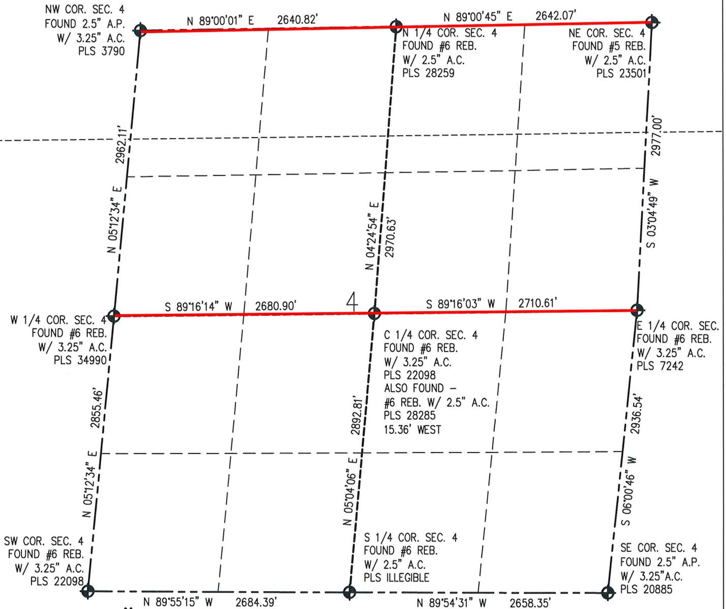
IN ACCORDANCE WITH A REQUEST FROM CRAIG RASMUSON - SYNERGY RESOURCES, BASELINE ENGINEERING CORP. HAS DETERMINED THE LOCATION OF THE SRC WEDEMAN A-5-3NHZ 1408' FNL AND 2438' FEL, AS MEASURED AT NINETY (90) DEGREES FROM THE SECTION LINE OF SECTION 5, TOWNSHIP 5 NORTH, RANGE 66 WEST AND THE BOTTOM HOLE LOCATION TO BE 1091' FNL AND 2149' FWL OF SECTION 3, TOWNSHIP 5 NORTH, RANGE 66 WEST, 6TH PRINCIPAL MERIDIAN, WELD COUNTY, COLORADO.
