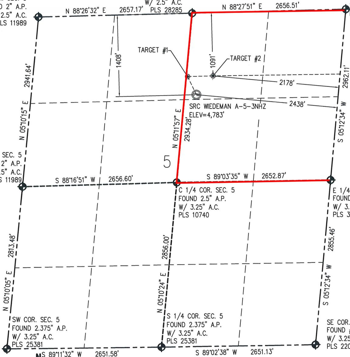
IN ACCORDANCE WITH A REQUEST FROM CRAIG RASMUSON - SYNERGY RESOURCES, BASELINE ENGINEERING CORP. HAS DETERMINED THE LOCATION OF THE SRC WIEDEMAN A-5-3NHZ TO BE 1408' FNL AND 2438' FEL, AS MEASURED AT NINETY (90) DEGREES FROM THE SECTION LINE OF SECTION 5, TOWNSHIP 5 NORTH, RANGE 66 WEST AND THE BOTTOM HOLE LOCATION TO BE 1091' FNL AND 2149' FWL OF SECTION 3, TOWNSHIP 5 NORTH, RANGE 66 WEST, 6TH PRINCIPAL MERIDIAN, WELD COUNTY, COLORADO.
