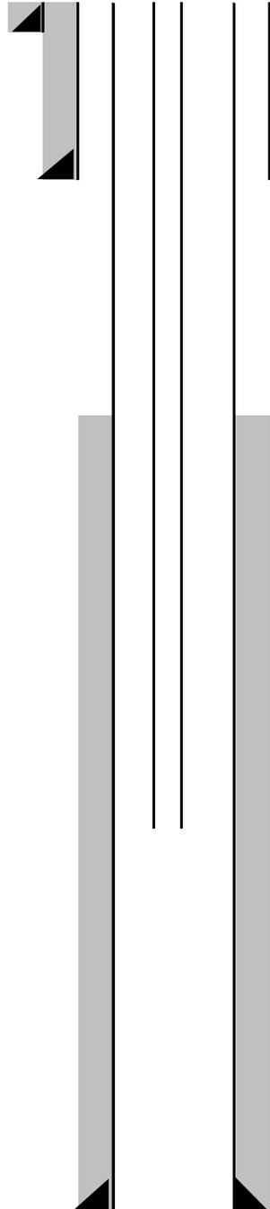
**Conductor 26" Hole 18" casing/liner 63' W/ 24 Sks cmt**
