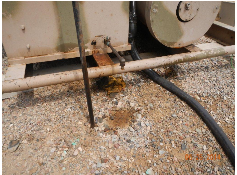
Soiled rags and staining at separators.
