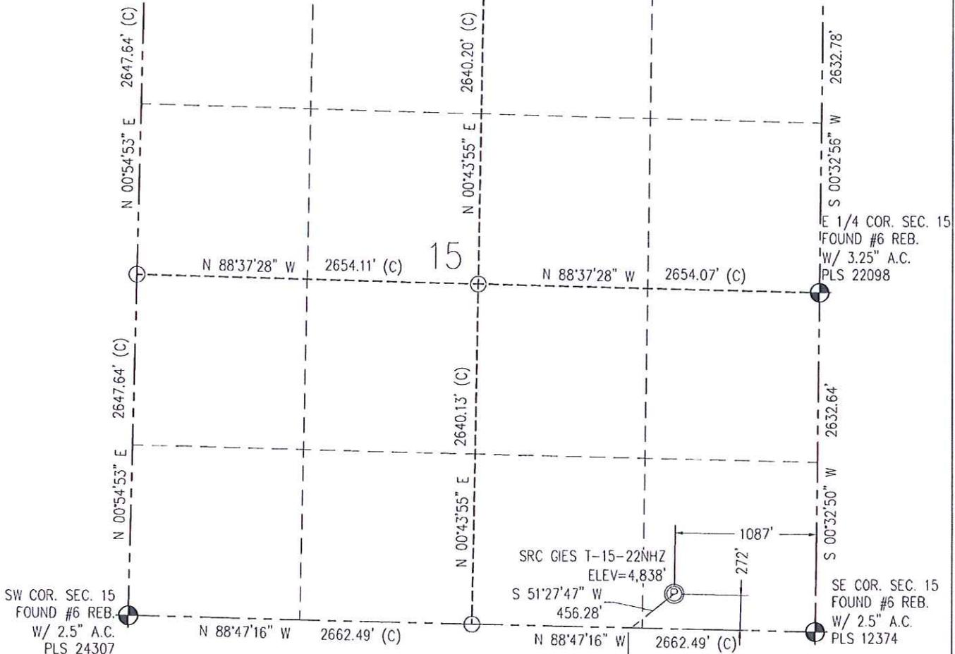
IN ACCORDANCE WITH A REQUEST FROM CRAIG RASMUSON - SYNERGY RESOURCES, BASELINE ENGINEERING CORP. HAS DETERMINED THE LOCATION OF THE SRC GIES T-15-22NHZ TO BE 272' FSL AND 1087' FEL, AS MEASURED AT NINETY (90) DEGREES FROM THE SECTION LINE OF SECTION 15, TOWNSHIP 7 NORTH, RANGE 65 WEST AND THE BOTTOM HOLE LOCATION TO BE 470' FSL AND 1424' FEL OF SECTION 22, TOWNSHIP 7 NORTH, RANGE 65 WEST, 6TH PRINCIPAL MERIDIAN, WELD COUNTY, COLORADO.
