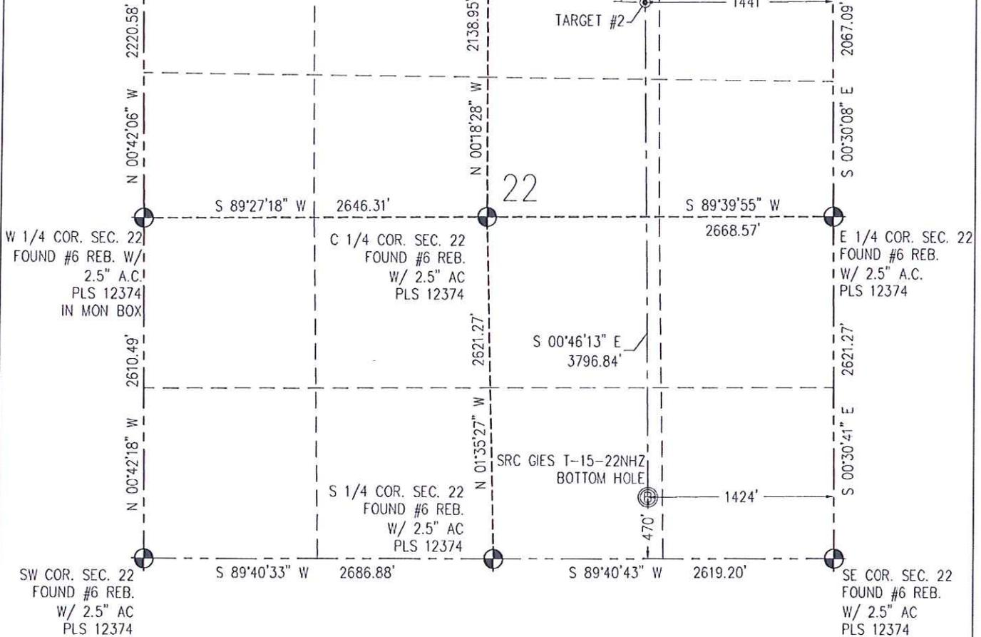
**N** IN ACCORDANCE WITH A REQUEST FROM CRAIG RASMUSON - SYNERGY RESOURCES, BASELINE ENGINEERING CORP. HAS DETERMINED THE LOCATION OF THE SRC GIES T-15-22NHZ TO BE 272' FSL AND 1087' FEL, AS MEASURED AT NINETY (90) DEGREES FROM THE SECTION LINE OF SECTION 15, TOWNSHIP 7 NORTH, RANGE 65 WEST AND THE BOTTOM HOLE LOCATION TO BE 470' FSL AND 1424' FEL OF SECTION 22, TOWNSHIP 7 NORTH, RANGE 65 WEST, 6TH PRINCIPAL MERIDIAN, WELD COUNTY, COLORADO.
