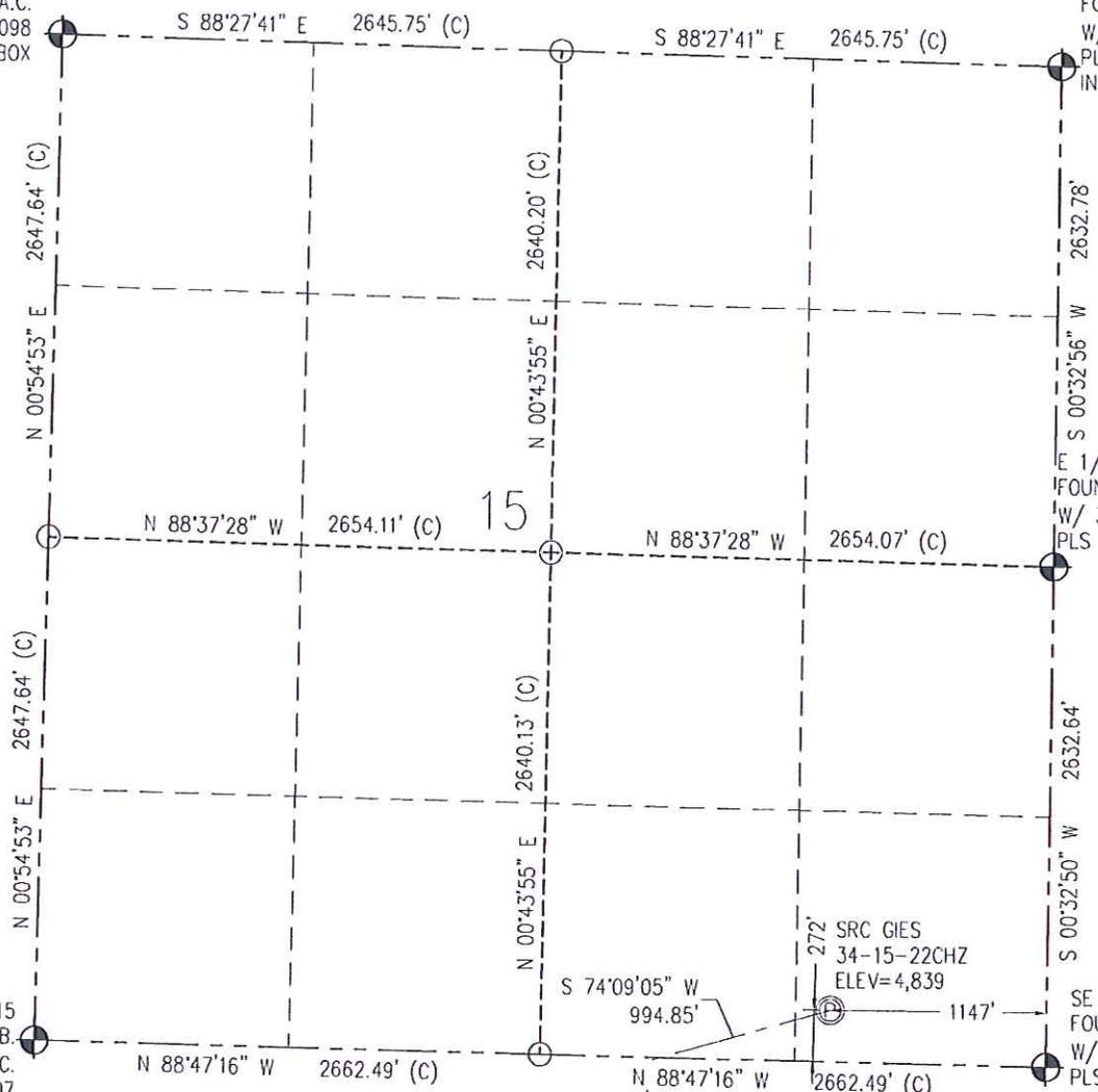
**N** IN ACCORDANCE WITH A REQUEST FROM CRAIG RASMUSON - SYNERGY RESOURCES, BASELINE ENGINEERING CORP. HAS DETERMINED THE LOCATION OF THE SRC GIES 34-15-22CHZ TO BE 272' FSL AND 1147' FEL, AS MEASURED AT NINETY (90) DEGREES FROM THE SECTION LINE OF SECTION 15, TOWNSHIP 7 NORTH, RANGE 65 WEST AND THE BOTTOM HOLE LOCATION TO BE 470' FSL AND 2084' FEL OF SECTION 22, TOWNSHIP 7 NORTH, RANGE 65 WEST, 6TH PRINCIPAL MERIDIAN, WELD COUNTY, COLORADO
