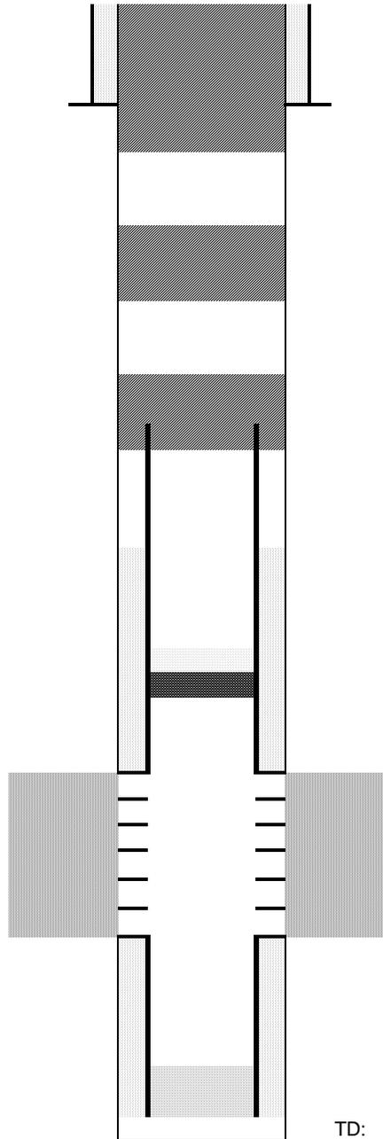
Cut surface casing off 6'-8' below surface.
