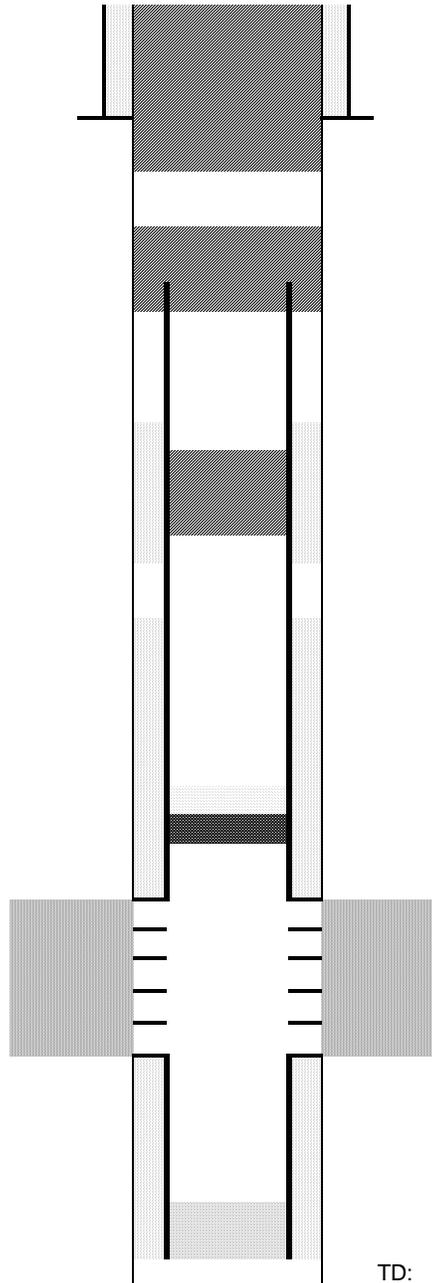
Cut surface casing off 6'-8' below surface.
