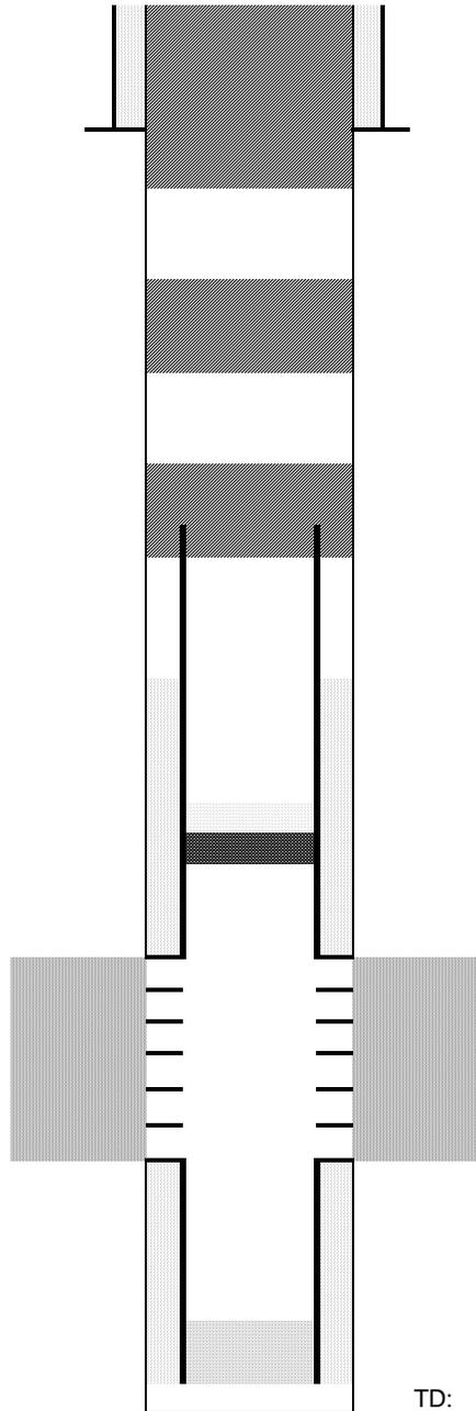
Cut surface casing off 6'-8' below surface.
