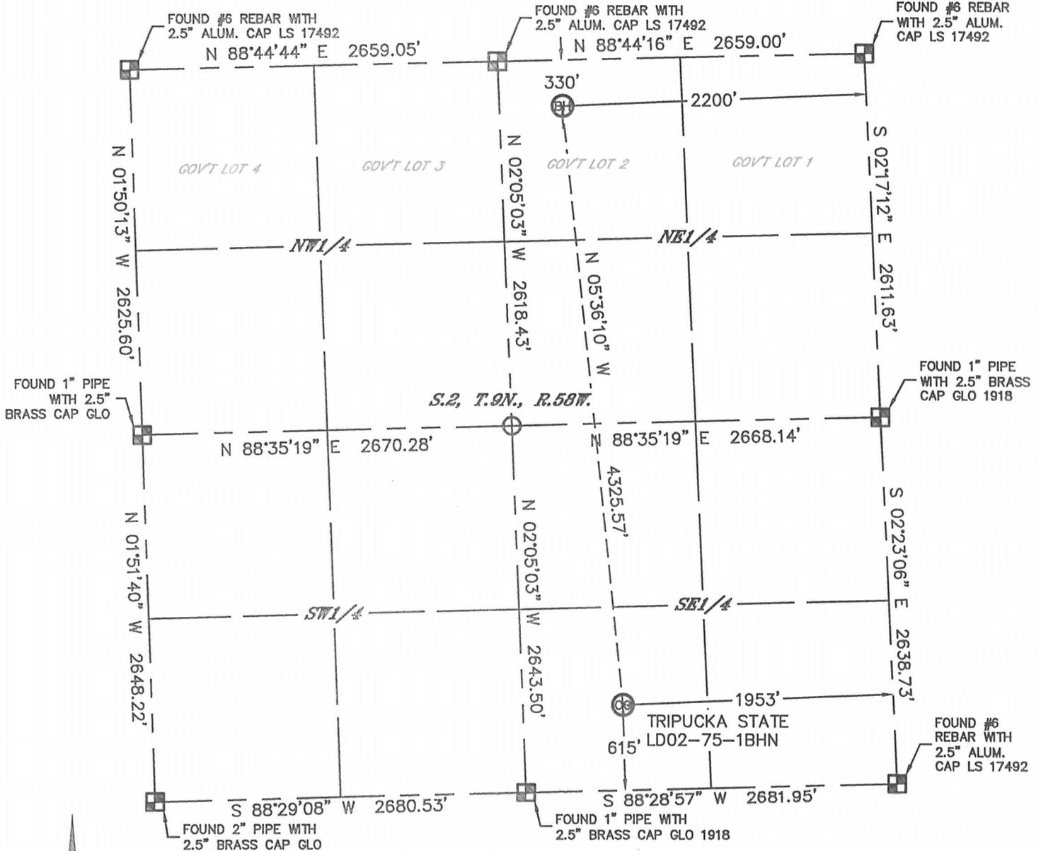
In accordance with a request from Cody Ball with Noble Energy Inc. Lat40°, Inc. has determined the surface location of the TRIPUCKA STATE LD02-75-1BHN to be 615' from the SOUTH line and 1953' from the EAST line and the bottom hole to be 330' from the NORTH line and 2200' from the EAST line as measured at right angles from the section lines of Section 2, Township 9 North, Range 58 West of the Sixth Principal Meridian, County of Weld, State of Colorado.
