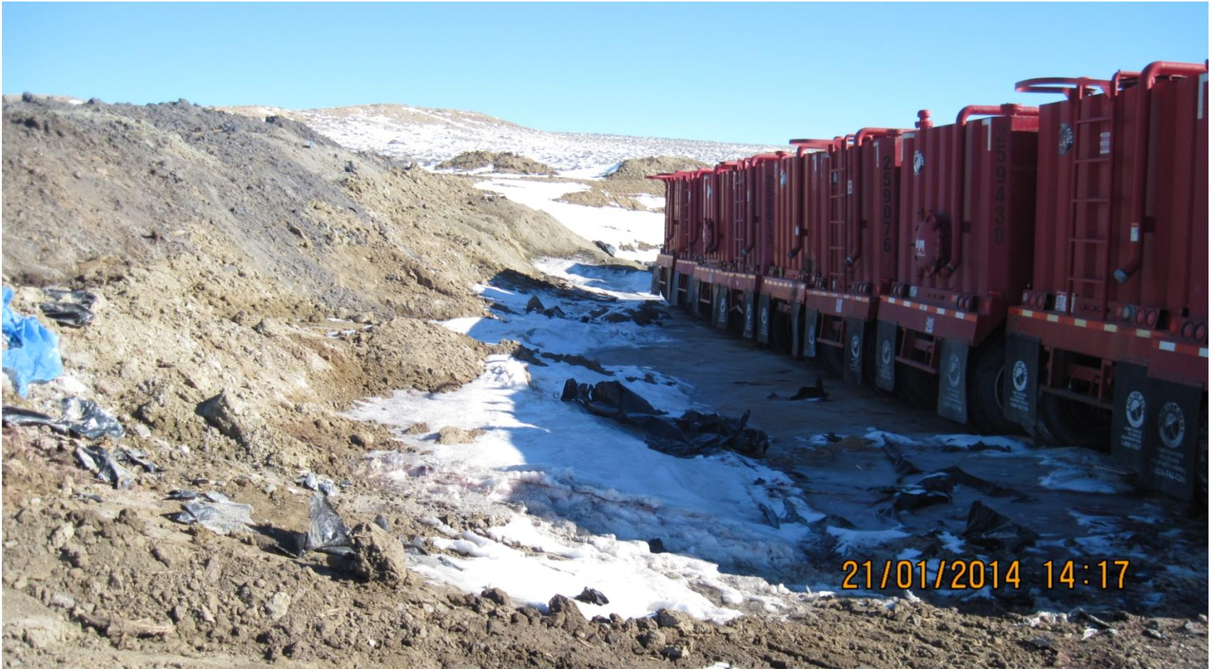
“Berm” that was installed since previous visit. Berm is not countinuous and frac tank is sitting in E&P waste.
