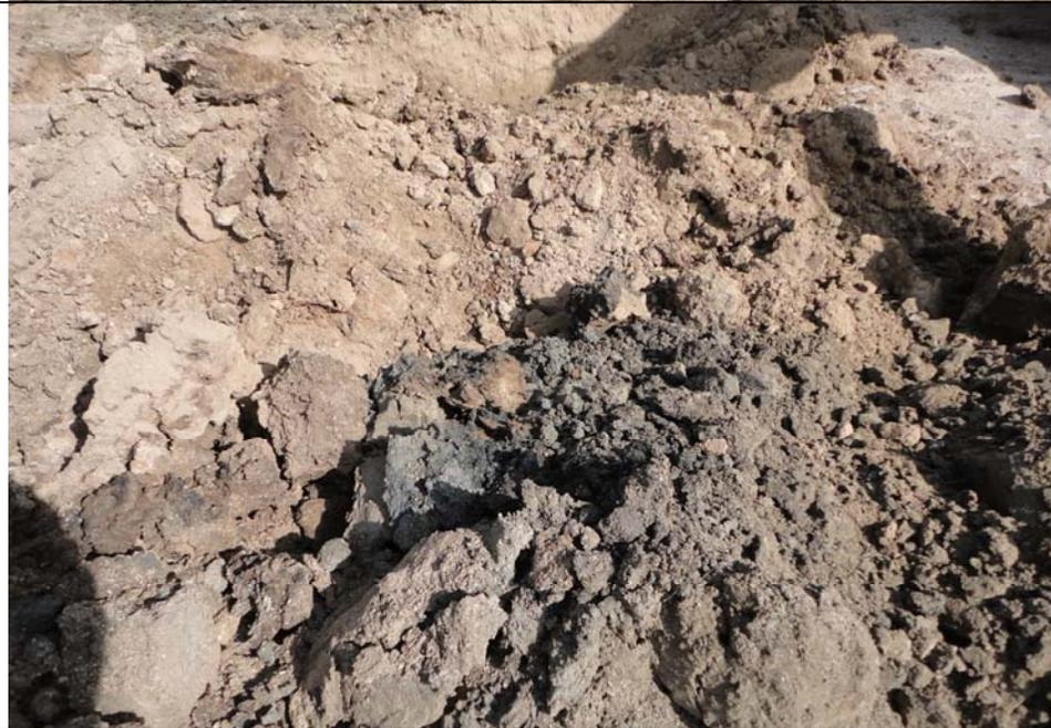
**Subject:** Photograph shows stained soils excavated from approximately 4.5 feet bgs in the west trench. Soils consisted of sandy clay to clayey silts.
