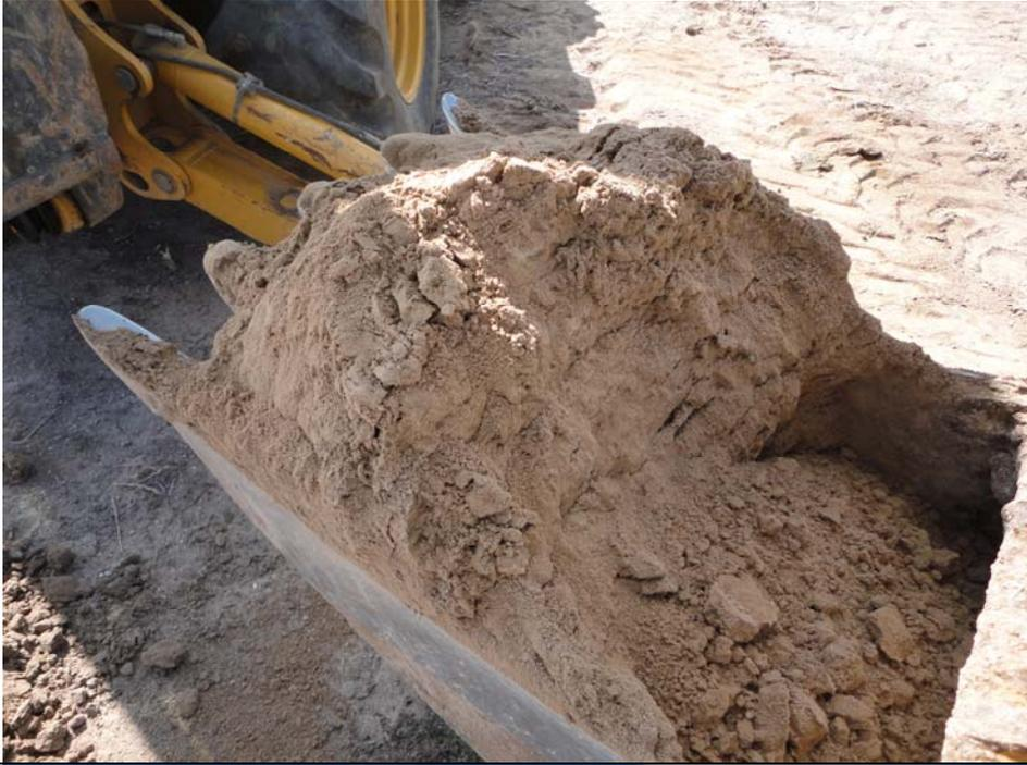
**Subject:** Impacted soils were not encountered in the trench excavated on the south side of the former skim pit. The soils did not exhibit signs of impact from the surface down to approximately 8 feet bgs. Soils consisted of sandy silt and silty clay.
