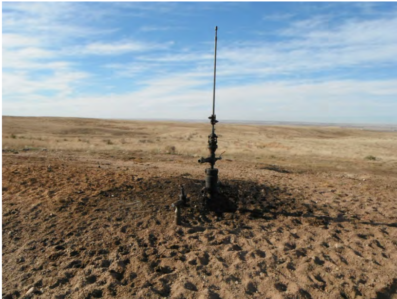
Wellhead after pump jack removal
