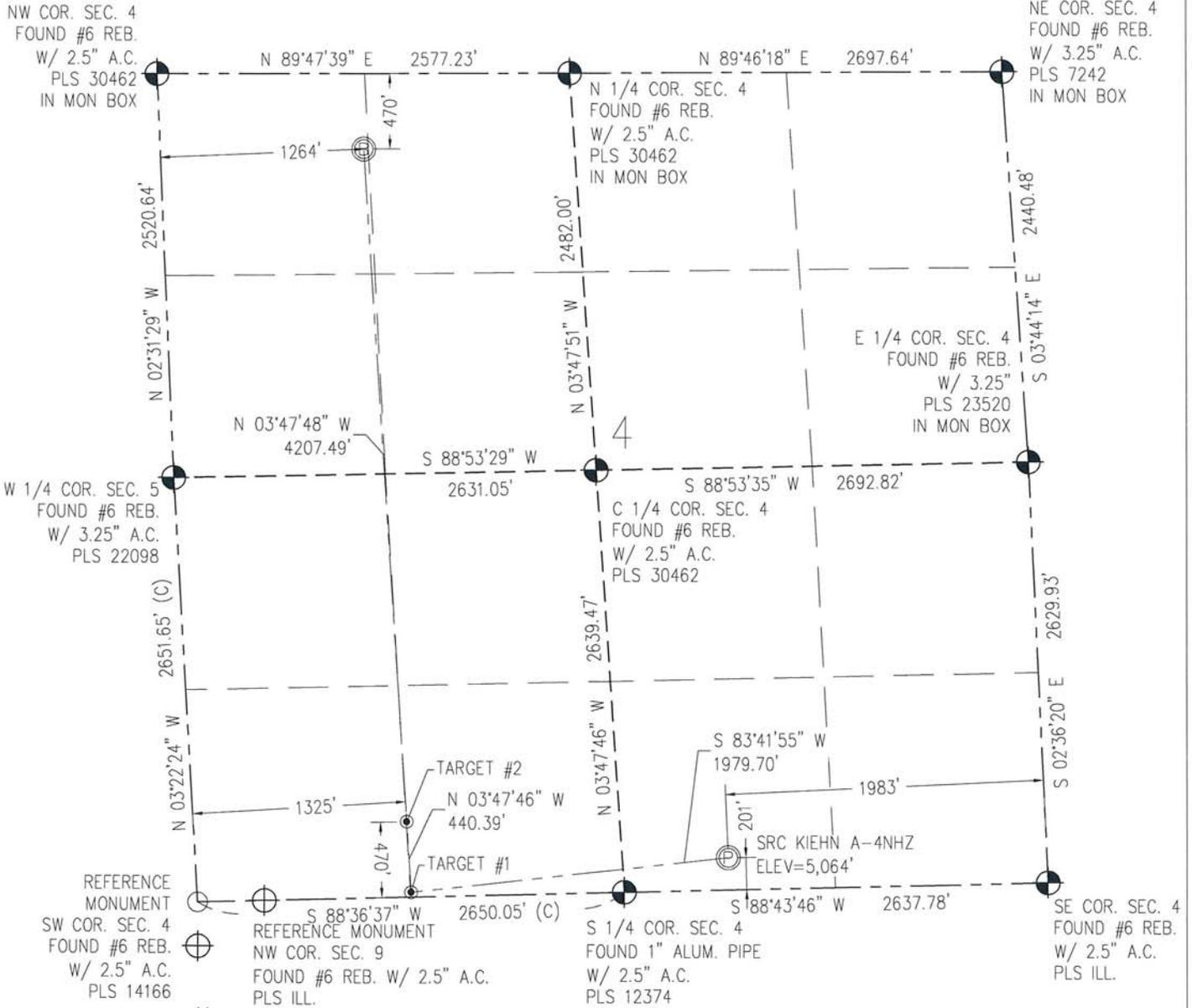
IN ACCORDANCE WITH A REQUEST FROM CRAIG RASMUSON - SYNERGY RESOURCES, BASELINE ENGINEERING CORP. HAS DETERMINED THE LOCATION OF THE SRC KIEHN A-4NHZ TO BE 201' FSL AND 1983' FEL, AS MEASURED AT NINETY (90) DEGREES FROM THE SECTION LINE OF SECTION 4, TOWNSHIP 4 NORTH, RANGE 68 WEST AND THE BOTTOM HOLE LOCATION TO BE 470' FNL AND 1264' FWL OF SECTION 4, TOWNSHIP 4 NORTH, RANGE 68 WEST, 6TH PRINCIPAL MERIDIAN, WELD COUNTY, COLORADO.
