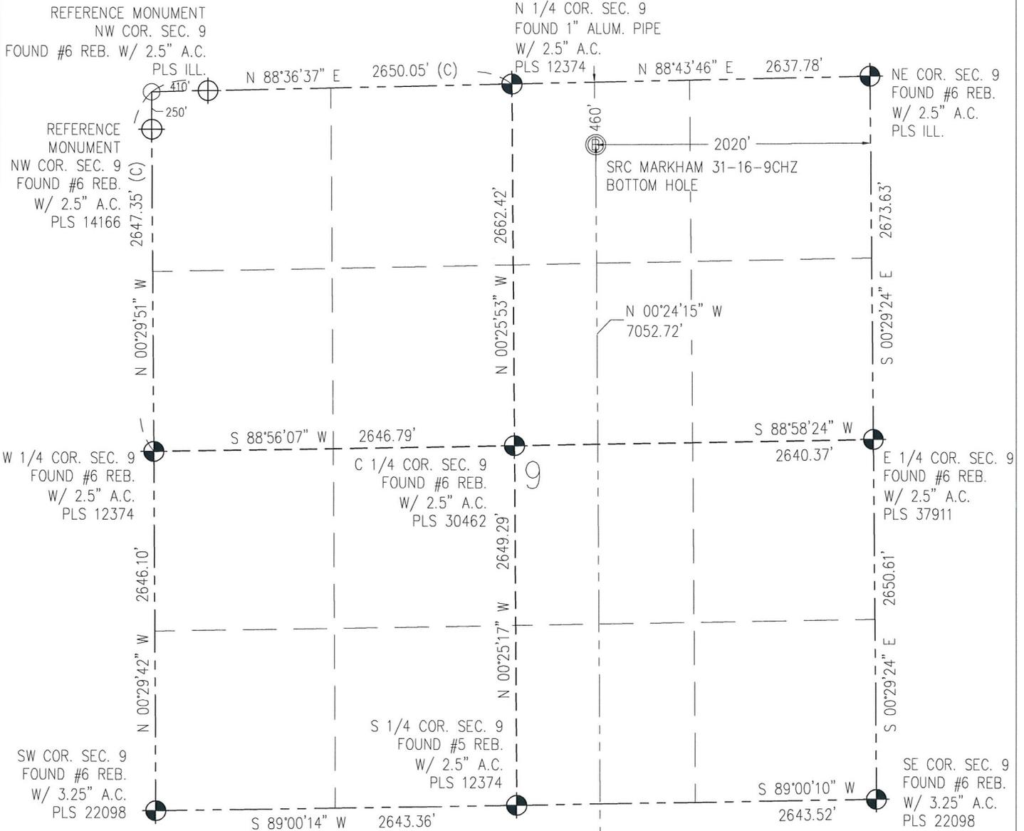
IN ACCORDANCE WITH A REQUEST FROM CRAIG RASMUSON - SYNERGY RESOURCES, BASELINE ENGINEERING CORP. HAS DETERMINED THE LOCATION OF THE SRC 31-16-9CHZ TO BE 2440' FNL AND 2032' FWL, AS MEASURED AT NINETY (90) DEGREES FROM THE SECTION LINE OF SECTION 16, TOWNSHIP 4 NORTH, RANGE 68 WEST AND THE BOTTOM HOLE LOCATION TO BE 460' FNL AND 2020' FEL OF SECTION 9, TOWNSHIP 4 NORTH, RANGE 68 WEST, 6TH PRINCIPAL MERIDIAN, WELD COUNTY, COLORADO.
