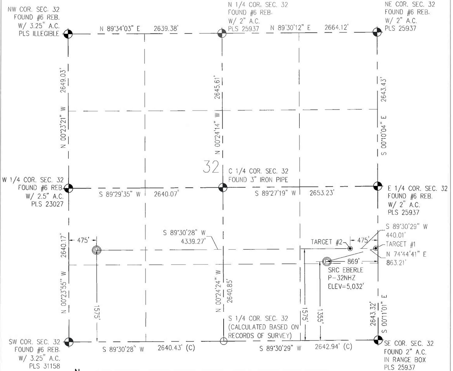
IN ACCORDANCE WITH A REQUEST FROM CRAIG RASMUSON - SYNERGY RESOURCES, BASELINE ENGINEERING CORP HAS DETERMINED THE LOCATION OF THE SRC EBERLE P-32NHZ TO BE 1355' FSL AND 869' FEL, AS MEASURED AT NINETY (90) DEGREES FROM THE SECTION LINE OF SECTION 32, TOWNSHIP 1 NORTH, RANGE 66 WEST AND THE BOTTOM HOLE LOCATION TO BE 1575' FSL AND 475' FWL OF SECTION 32, TOWNSHIP 1 NORTH, RANGE 66 WEST, 6TH PRINCIPAL MERIDIAN, WELD COUNTY, COLORADO.
